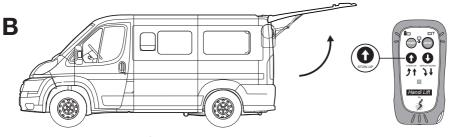
B. Press and hold the button **()** to open the hatch door.
