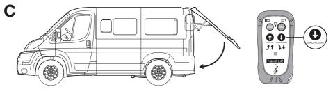
C. Press and hold the button **U** to close the hatch door.
